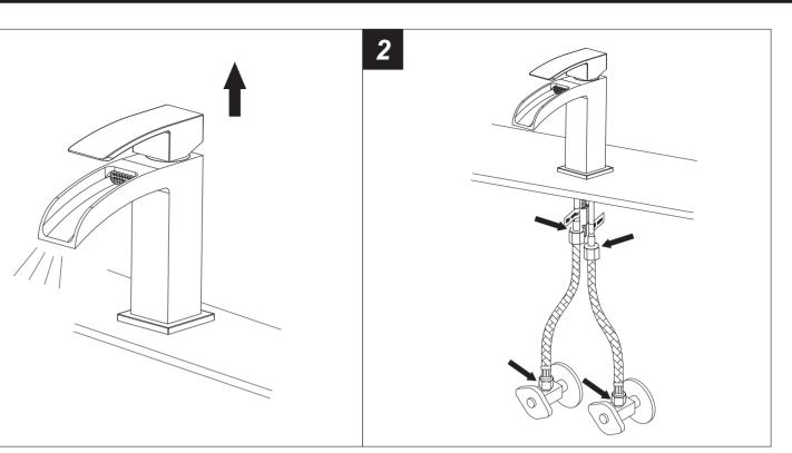
1. Turn the faucet handle all the way on, turn on hot and cold water supply and flush water lines for one minute. 2. Check all connections at arrows for leaks, re-tighten it if necessary. .
